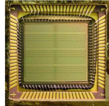
1995 – GBT Spectrometer Chip, 1024 Lags, 125 MHz Clock, \$200
